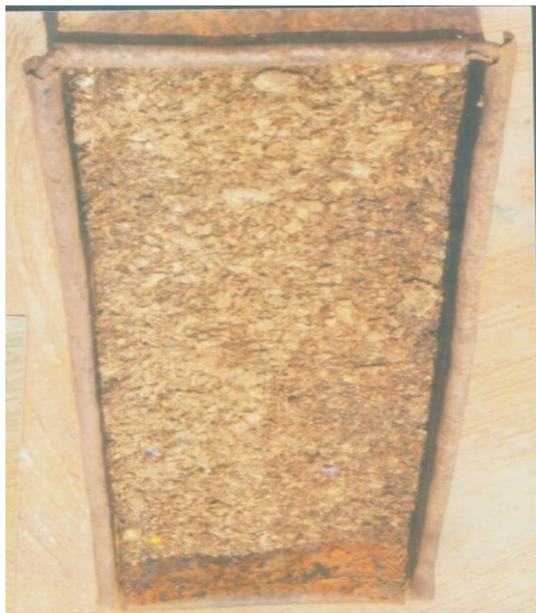
Fig 2.2 Briquette produced Groundnut Shell with Binder (After Compression) Fig 3.3 Picture of the Bottle Jack briquette Machine
