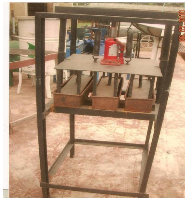
Fig 2.2 Briquette produced Groundnut Shell with Binder (After Compression) Fig 3.3 Picture of the Bottle Jack briquette Machine
